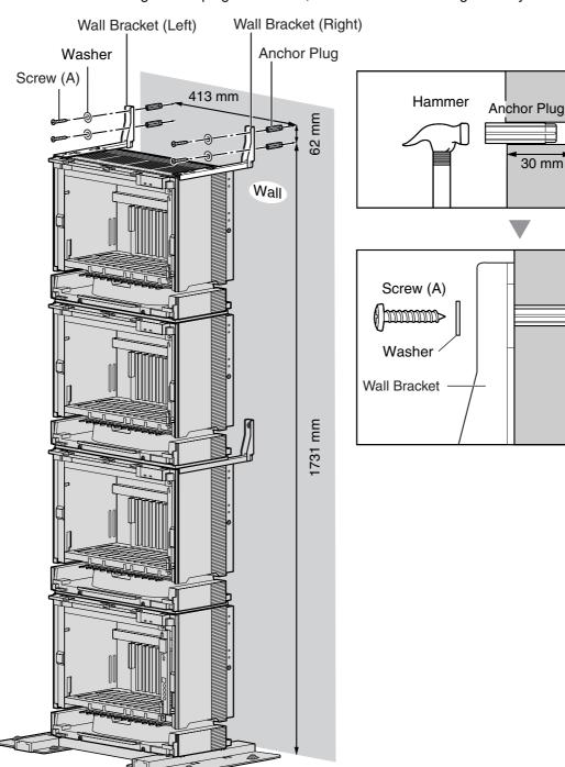
2. Check that the shelves are standing exactly vertically. If the upper shelves are leaning slightly to one side, move Expansion Shelf 3 to adjust the position. (Since the wall brackets are attached loosely to Expansion Shelf 3, it should be possible to adjust the position of the shelves.)
