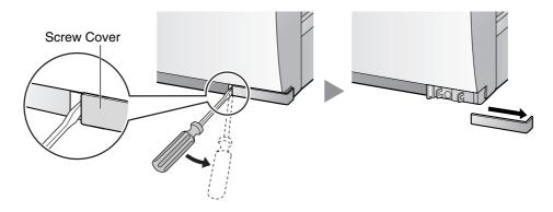
2. Turn the screw anticlockwise to loosen.
