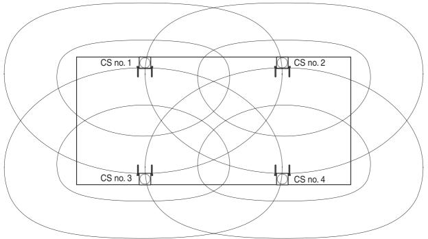
c. Make sure that the radio signal strength level is greater than "3" at any location in the service area required by the user.
