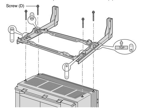
**3.** Install 4 anchor plugs in the wall, using the wall brackets as a template. Fix the wall brackets to the wall with 4 screws (A).
