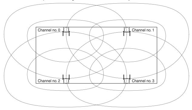
Make sure that the radio signal strength level is greater than "3" at any location in the service area required by the user.
