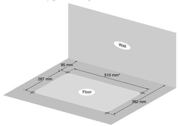
\* If the direction of the base stands is reversed, the measurement must be 443.4 mm.
