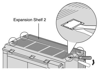
2. Fix the metal bracket to Expansion Shelf 2 with 4 screws (B).
